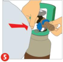
If using foil inflator, hold neck of balloon over nozzle and push back, release when balloon is inflated to correct size.
