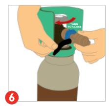
After inflation close cylinder valve then push tip to release surplus gas.
